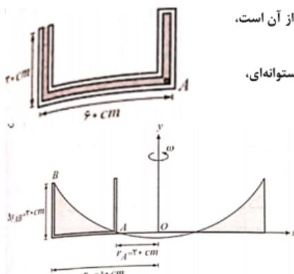
$$\Delta y_{BA} = \frac{\omega^2}{2g} (r_B^2 - r_A^2) \gamma \longrightarrow 0.3 = \frac{\omega^2}{2 \times 10} (0.8^2 - 0.2^2) \longrightarrow \omega = \sqrt{10} \text{ rad/s}$$
