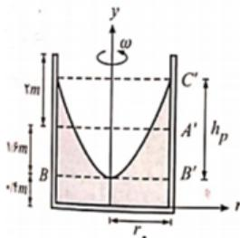
$$h_p = \frac{\omega^2 r_0^2}{2g} = 8^2 \times \frac{1^2}{2 \times 10} = 3.2 \text{ m}$$
