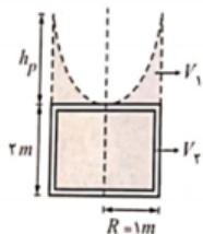
$$h_p = \frac{\omega^2 r_0^2}{2g} = \frac{10^2 \times 1^2}{2 \times 10} = 5 \text{ m}$$
