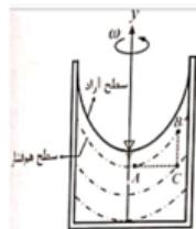
$$P_A = P_B \longrightarrow P_0 + \gamma \left( \frac{\omega^2 r_A^2}{2g} \right) - \gamma y_A = P_0 + \gamma \left( \frac{\omega^2 r_B^2}{2g} \right) - \gamma y_B$$
