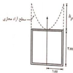
$$F_{کف} = \gamma V = 8 \left[ \pi \times 1^2 \times 2 + \frac{1}{2} \pi \times 1^2 \times 5 \right] = 36\pi \text{ kN}$$
