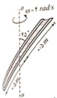
$$h_p = \frac{\omega^2 r_0^2}{2g} = \frac{4^2 \times (0.5 \times \cos 45)^2}{2 \times 10} = 0.1 \text{ m}$$
